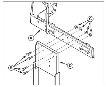
Figure 3. Install Hitch Assembly
